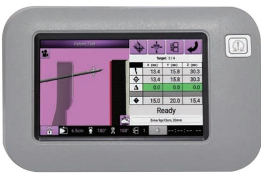
Automate calculations – biopsy needle parameters are programmed into the system to display safety margins and relevant distance in real-time.
